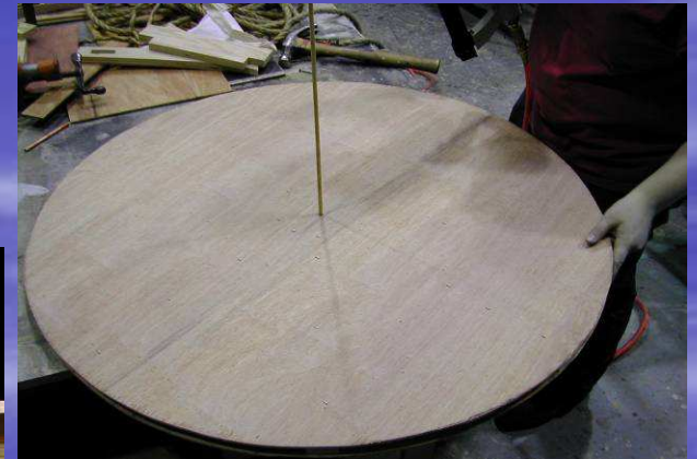
We mounted the china silk column to the smaller wheel, which was 3' in diameter and was built out of 1x2 and Luan sheets in order to reduce the weight.
